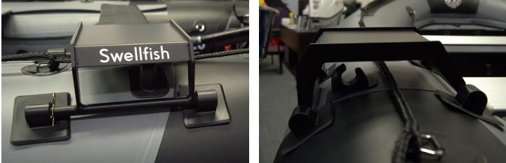
**Step Five** Prepping for the glue up. Once you are happy with the placement, temporarily tape the four glue-on pads to the boat. This will allow you to check the fit with the glue-on pads staying where you have placed them.
