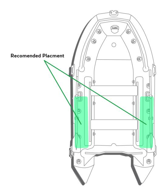
**Step Four** The downrigger mount should slightly overhang the center tube, ensuring the top mounting surface is level. The longer bar with the R-Clip must be on the boat's outside and towards the bow. The short bars point towards the transom.
