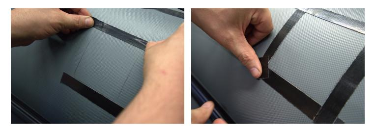
**Step Seven** Gluing on the pads. We recommend using either Stabond UK-148 or RH Adhesives HH-66. Following the glue's instructions, glue the mount to the boat. Both require 24hrs for full-strength adhesion.
