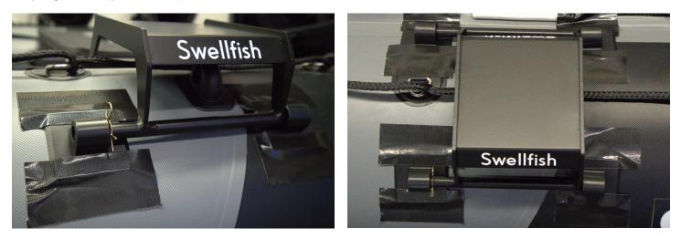
To check the fit and placement of the pads, remove the R-Clip before removing the mount to ensure it can be easily reattached. If you're satisfied that the mount can be unclipped and removed when not in use, proceed to the next step.
