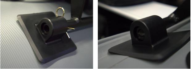
**Step Three** To ensure proper placement, temporarily place the mount on the boat in the approximate place where you will want it. The mount should be positioned on the tube between the center of the boat and the transom. However, it is important to adjust the placement based on your own comfort and needs while on the water. Keep in mind that each person and setup may require a unique placement.
